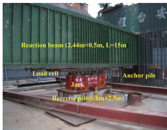
Fig. 1 Arrangement of the test setup of the C2 shaft
