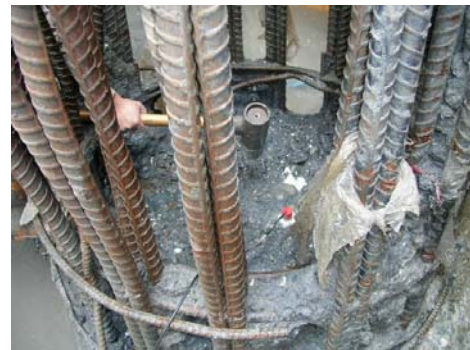
Fig. 11 Sonic echo testing
