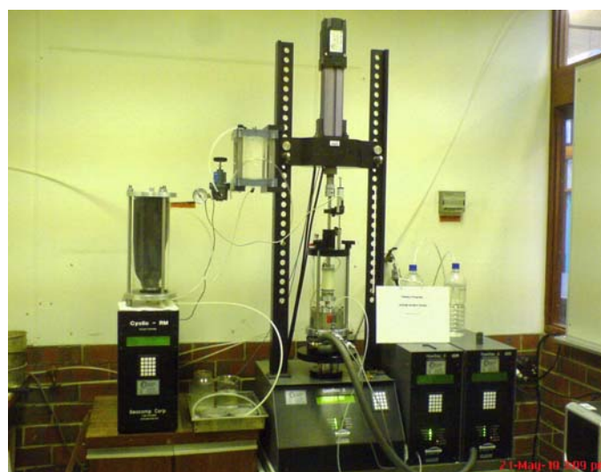
Fig. 1 Static/cyclic loading triaxial system
