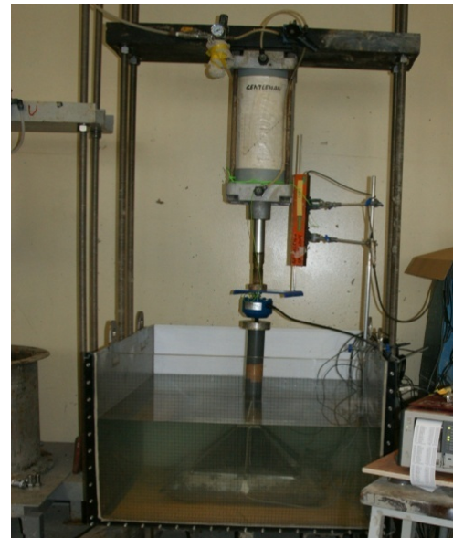
Fig. 2 Geotextile bag loading test apparatus
