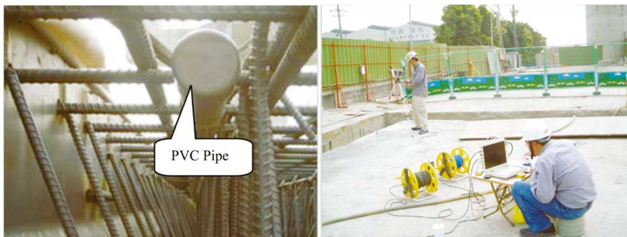
Fig. 5 PVC test pipe in the diaphragm wall and the ultrasonic test
