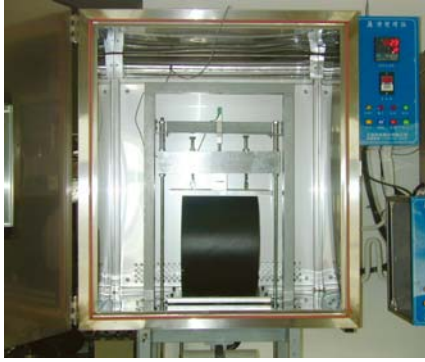
Fig. 2 Setup of the accelerated pipe stiffness test apparatus
