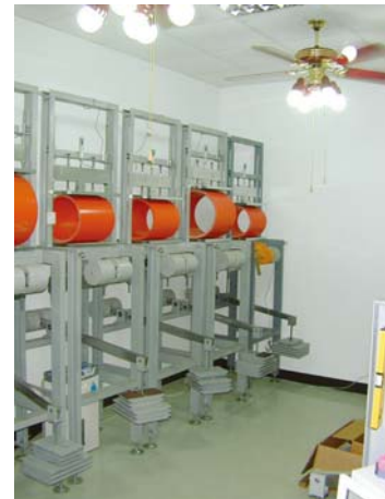
Fig. 1 Setup of the long-term pipe stiffness test apparatuses
