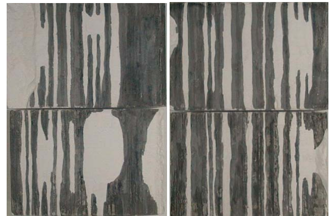
(b) 1/2 division, specimen length = 150 mm
