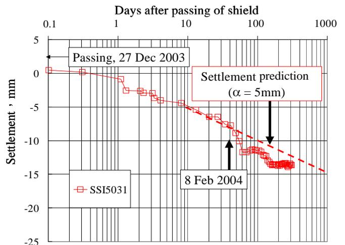
Fig. 17 Analyses of settlement, SSI5031, Section 0210B
