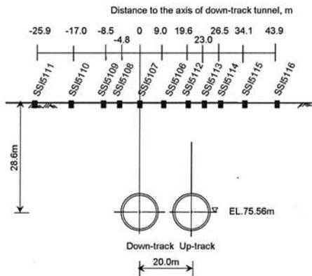
(a) Layout of instruments, Section 0246A
