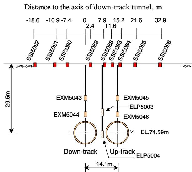
Fig. 2 Layout of instruments, Section 0128B
