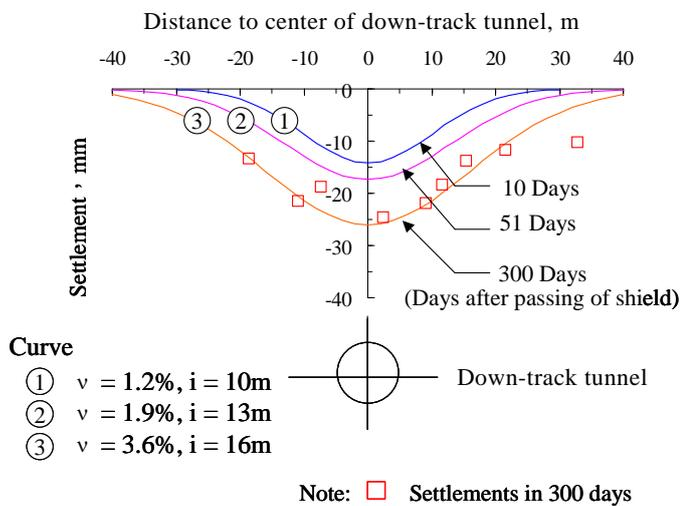
Fig. 9 Idealized settlement troughs, Section 0128B
