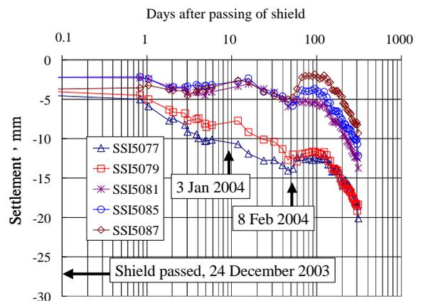
Fig. 11 Ground settlements, Section 0175A
