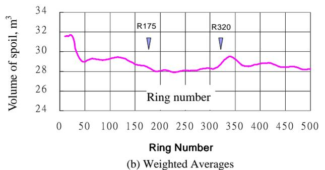
Fig. 18 Quantity of spoil discharged from tunnel
