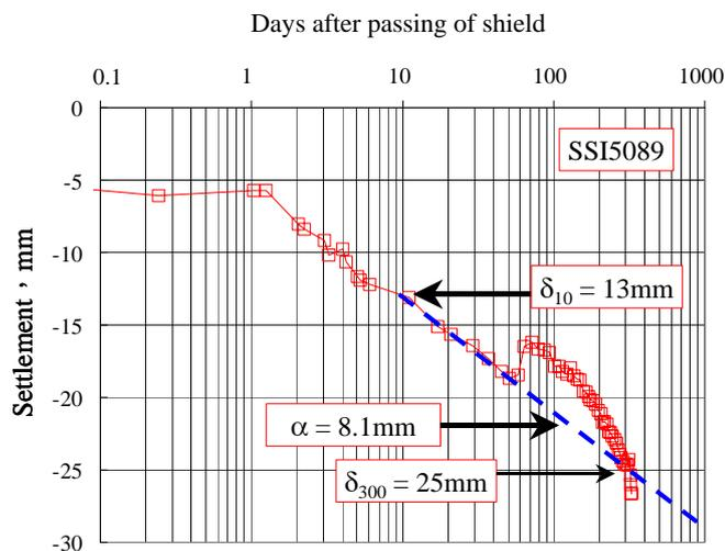
Fig. 15 Analyses of settlement, SSI5089, Section 0128B
