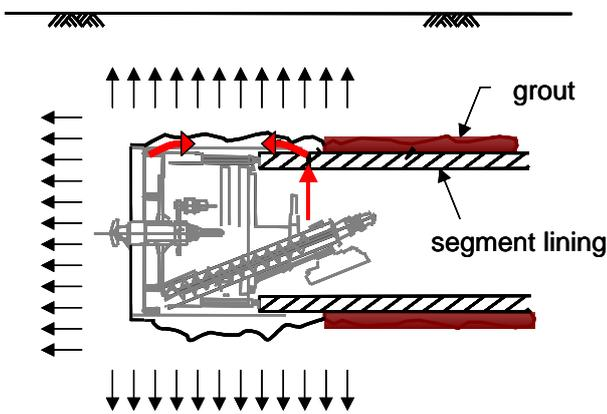
Fig. 23 Mechanism of ground heave
