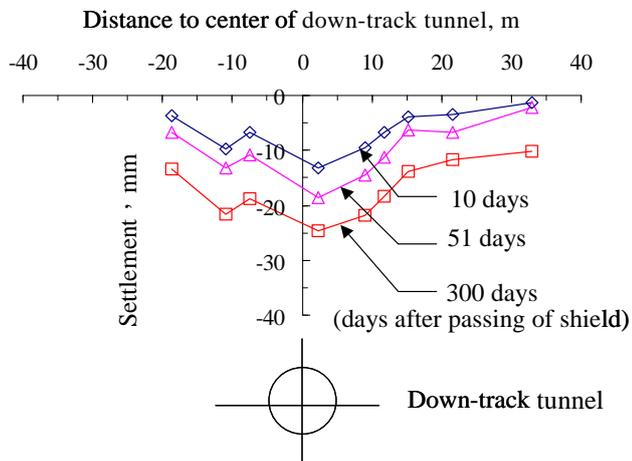
Fig. 8 Settlement troughs, Section 0128B
