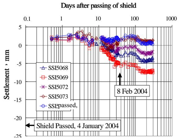
Fig. 10 Ground settlements, Section 0285B
