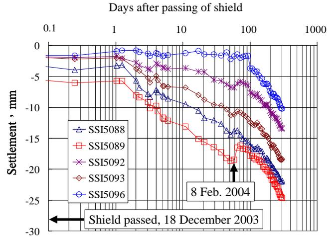
Fig. 6 Ground settlements, Section 0128B
