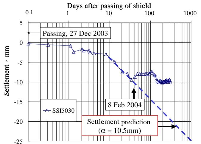
Fig. 16 Analyses of settlement, SSI5030, Section 0210B
