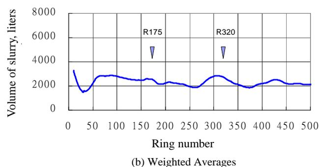
Fig. 19 Quantity of slurry injected into earth chamber
