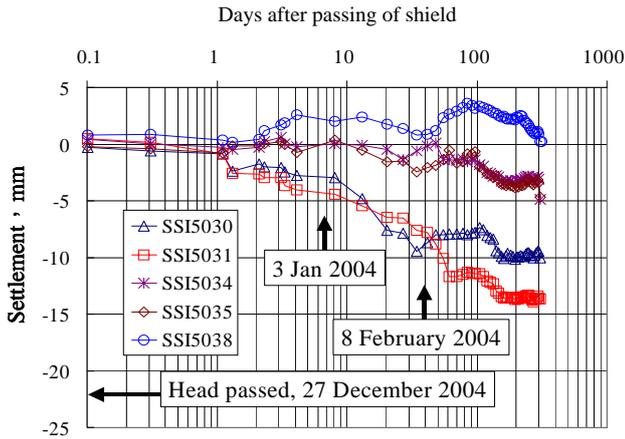
Fig. 12 Ground settlements, Section 0210B
