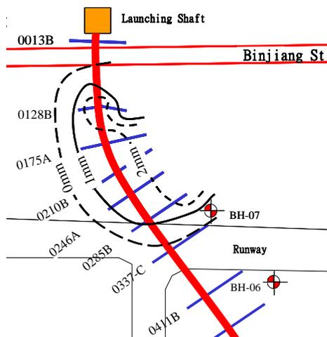
Fig. 14 Ground heave observed between 1 Feb. and 31 May, 2004
