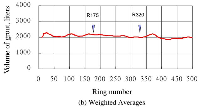
Fig. 20 Quantity of grout injected at the tail of shield
