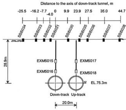
(a) Layout of instruments, Section 0210B
