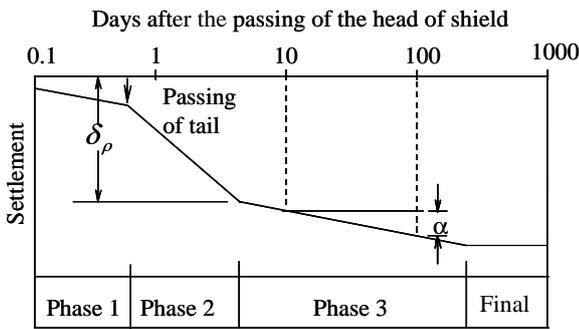
Fig. 5 Logarithmic model for simulating settlement curves
