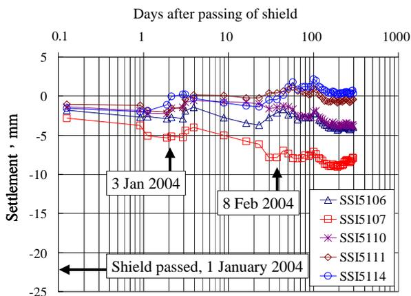
Fig. 13 Ground settlements, Section 0246A
