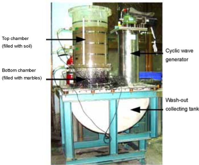
Fig. 4 Photo of cyclic flow apparatus (Ho, 2007)
