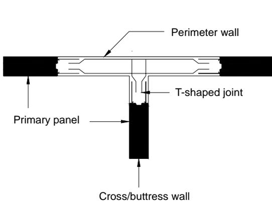
**Fig. 6 Schematic diagram of a rigid T-shaped joint**
