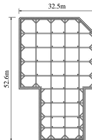
Fig. 1 Plan layout of retaining system
