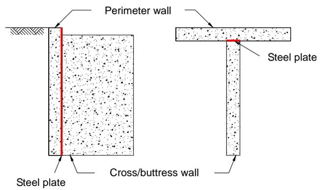
**Fig. 7 Schematic diagram of a clean contact joint**
