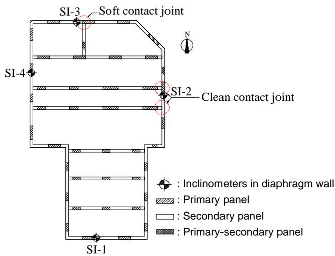
**Fig. 5 Panel layout of perimeter and cross walls**
