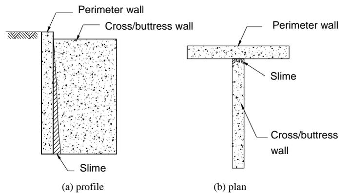
**Fig. 8 Schematic diagram of a soft contact joint**
