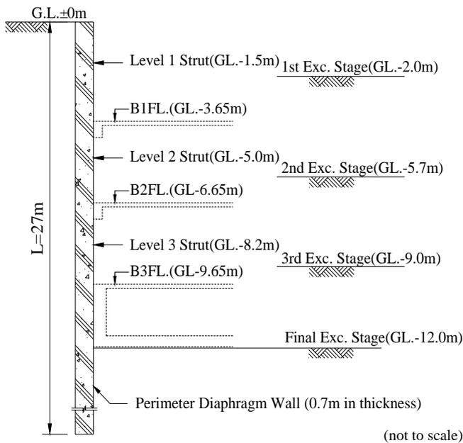
Fig. 2 Profile of retaining system
