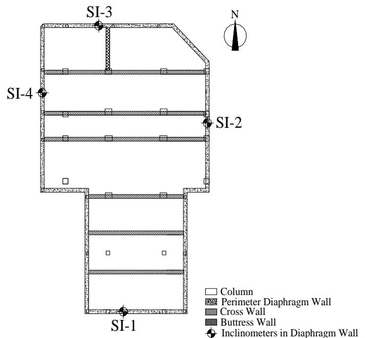
Fig. 3 Plan layout of cross/buttress walls
