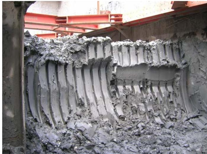
**Fig. 4 Silty clay of the construction site at GL.-10 m**
