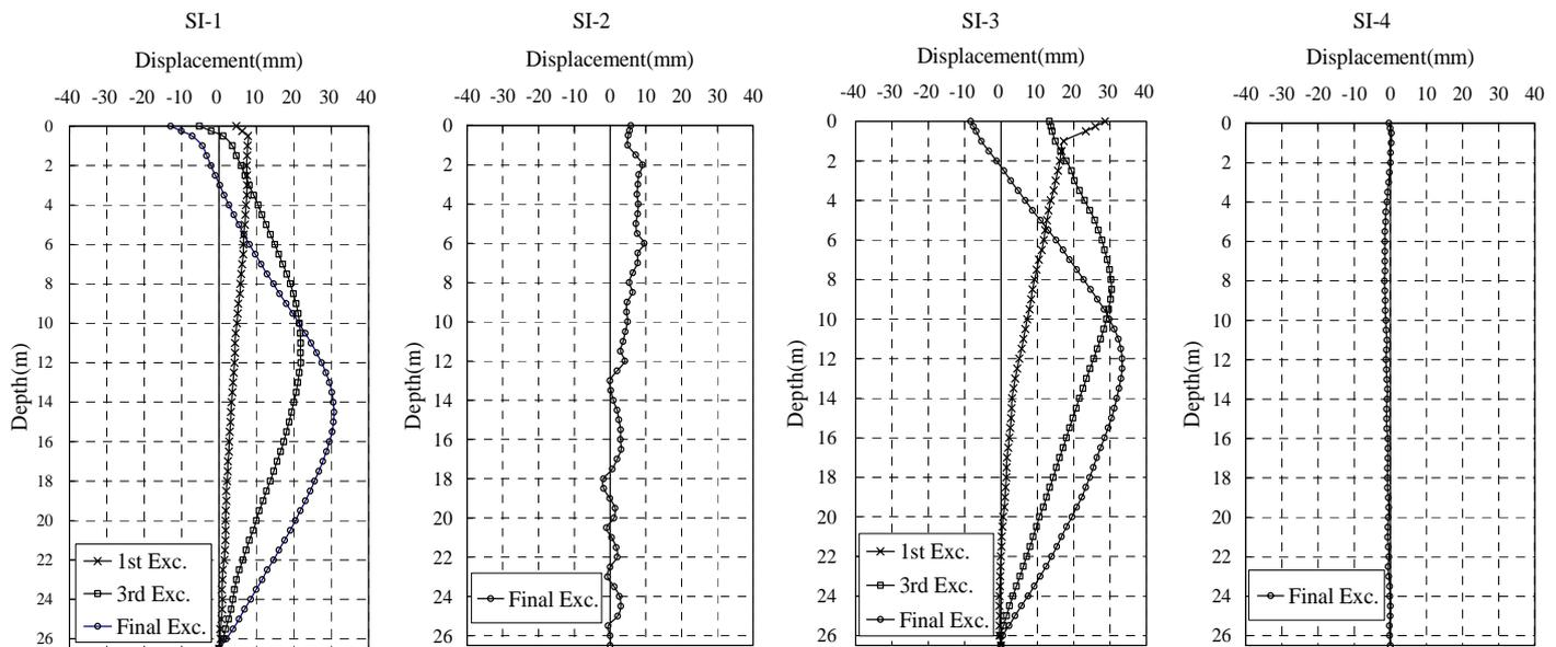
**Fig. 9 Displacement curves of perimeter diaphragm wall (1st, 3rd and final excavation stages for SI-1, 3)**
