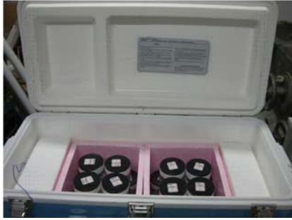
(b) A well-insulated container for suction equilibrium
