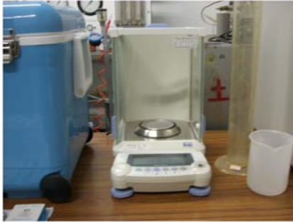
(d) Using a balance at least to the nearest 0.1 mg accuracy
