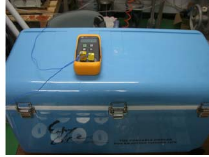
(c) Monitoring temperature of container during suction equilibrium
