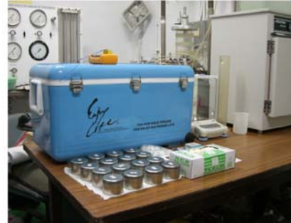
(e) Soil suction measurement set up
