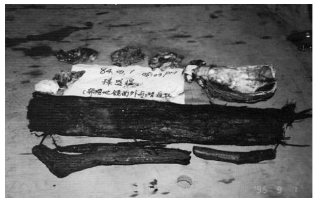
Fig. 16 Drift wood obtained between diaphragm wall and shield machine
