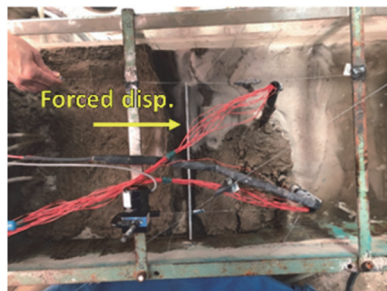
(d) Forced displacement by a penetrated aluminum sheet to approximate a large lateral spreading displacement
