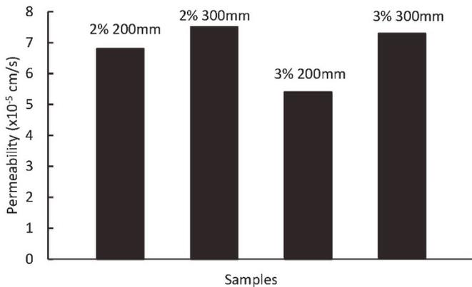
**Fig. 5 Variation of hydraulic conductivity for different mixes**
