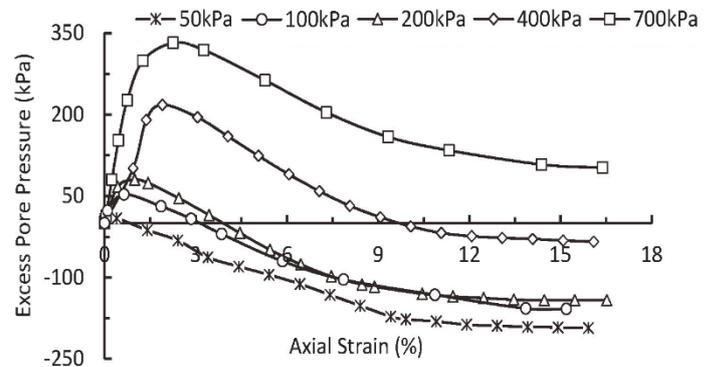
**Fig. 7 Variation of excess pore pressure with axial strain for all the confining pressures**
