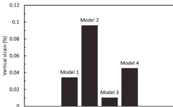
**Fig. 16 Comparison of the vertical strains developed at the crown of the pipe for different models**
