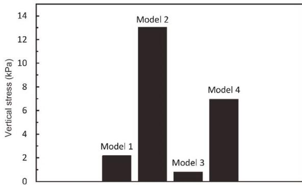
**Fig. 15 Comparison of the vertical stresses developed at the crown of the pipe for different models**
