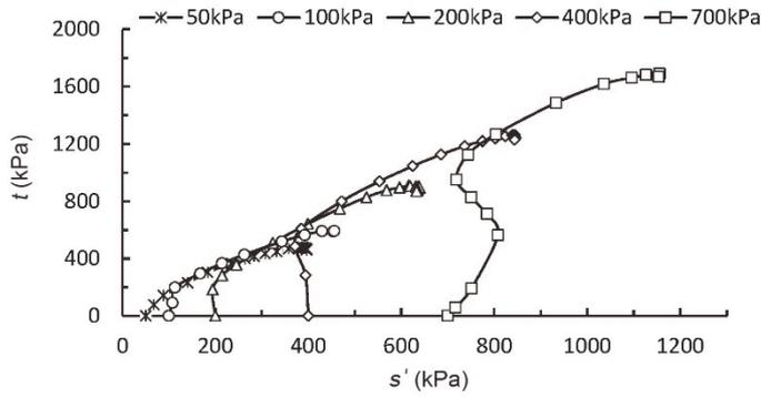
**Fig. 8** Effective stress paths obtained for all the confining pressures
