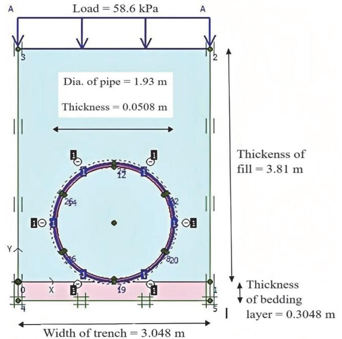
**Fig. 10 Finite element model considered for all the analyses**
