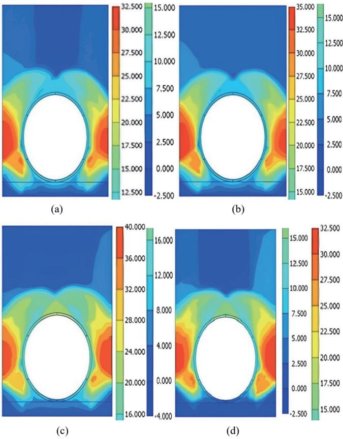
**Fig. 12** Plot of total displacements (in mm) for (a) Model 1; (b) Model 2; (c) Model 3; and (d) Model 4
