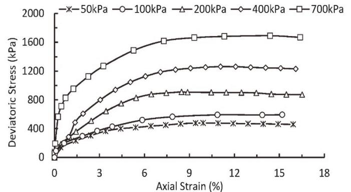
**Fig. 6 Observed deviatoric stress-axial strain variation for all the confining pressures**
