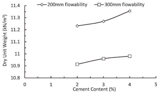
**Fig. 4 Dry unit weight variation for different flowable fill mixes**
