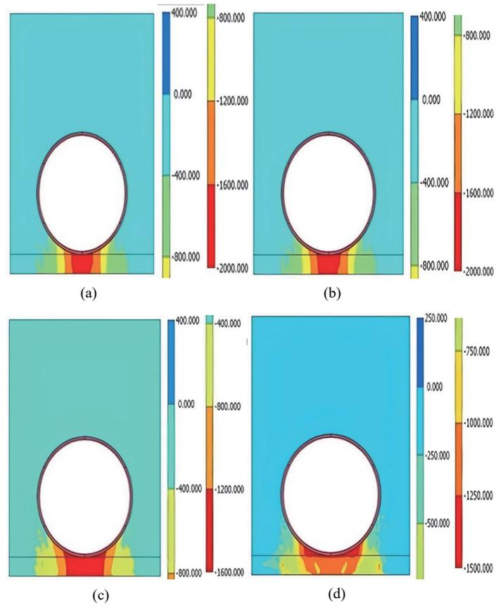
**Fig. 14** Plot of effective stresses (in kPa) for (a) Model 1; (b) Model 2; (c) Model 3; and (d) Model 4
