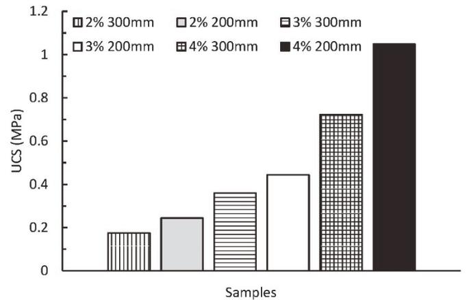
Fig. 3 UCS values at 28 days for different samples
