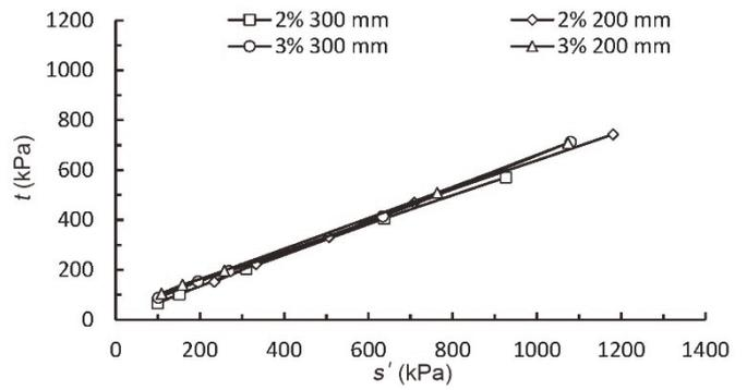
**Fig. 9** Modified failure envelopes for different conditions for peak values of  $\sigma'_1 / \sigma'_3$  for flowable fill sample
