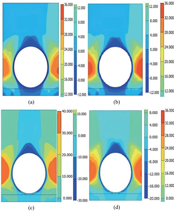
**Fig. 13** Plot of vertical displacement (in mm) for (a) Model 1; (b) Model 2; (c) Model 3; and (d) Model 4
