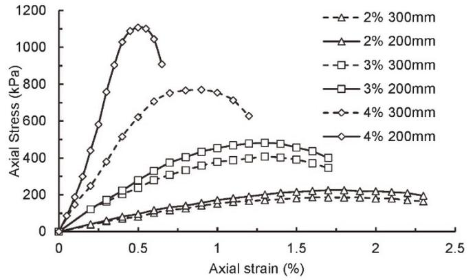
Fig. 2 Stress-strain variation for varying cement contents
