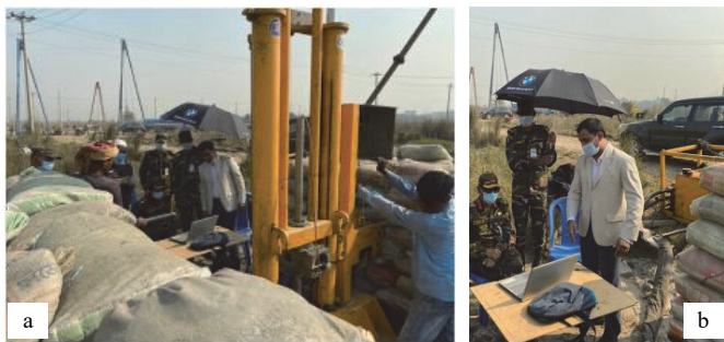
Fig. 2 Cone penetration test at soil site
