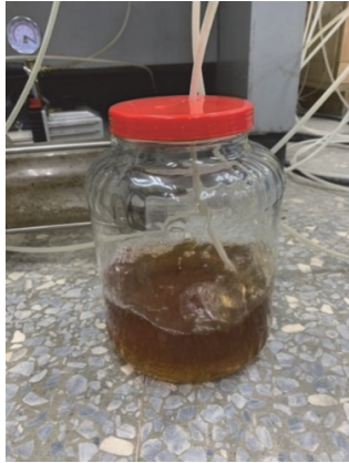
Fig. 3 24-hours air pumping for soil improvement solution
