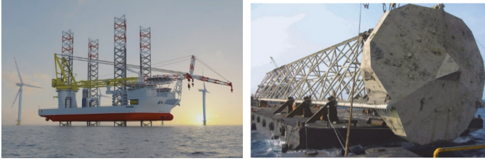
(a) Jack-up barge (from Durakovi 2020) (b) Spudcan foundation (form Pisanò et al. 2019)
