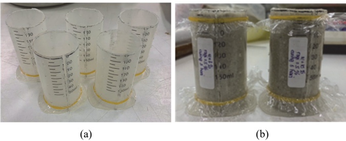
Fig. 3 The photos of (a) cylindrical mold and (b) sample after casted into the mold
