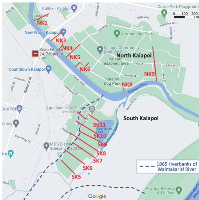
Fig. 7 Survey lines for surface displacement caused by lateral spreading in Kaiapoi during 2010-2011 Canterbury earthquake sequence (after Robinson 2016 and Wotherspoon et al. 2012; base map provided by Google Map)
