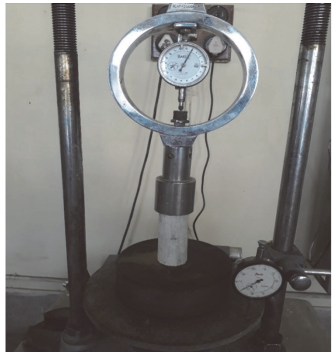
Fig. 5 Unconfined compressive strength test of biocemented sand
