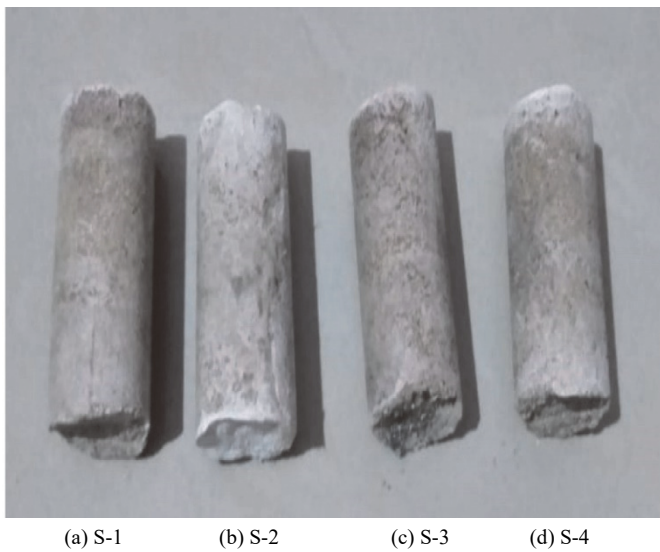
Fig. 4 Sand after MICCP treatment with different concentrations of soluble calcium and urea
