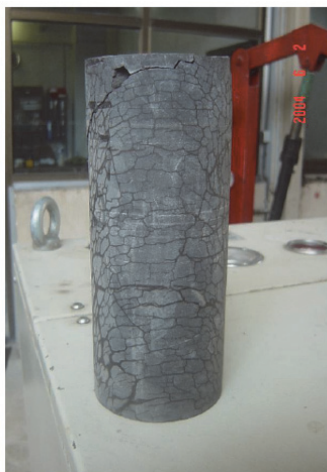
(b) A shale sample after performing a swelling test
