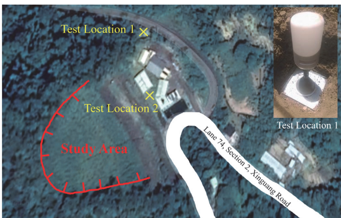
Fig. 6 Locations of sand-cone test (Google map)
