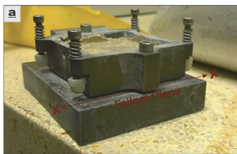
(a) Compacted specimen in shear box
